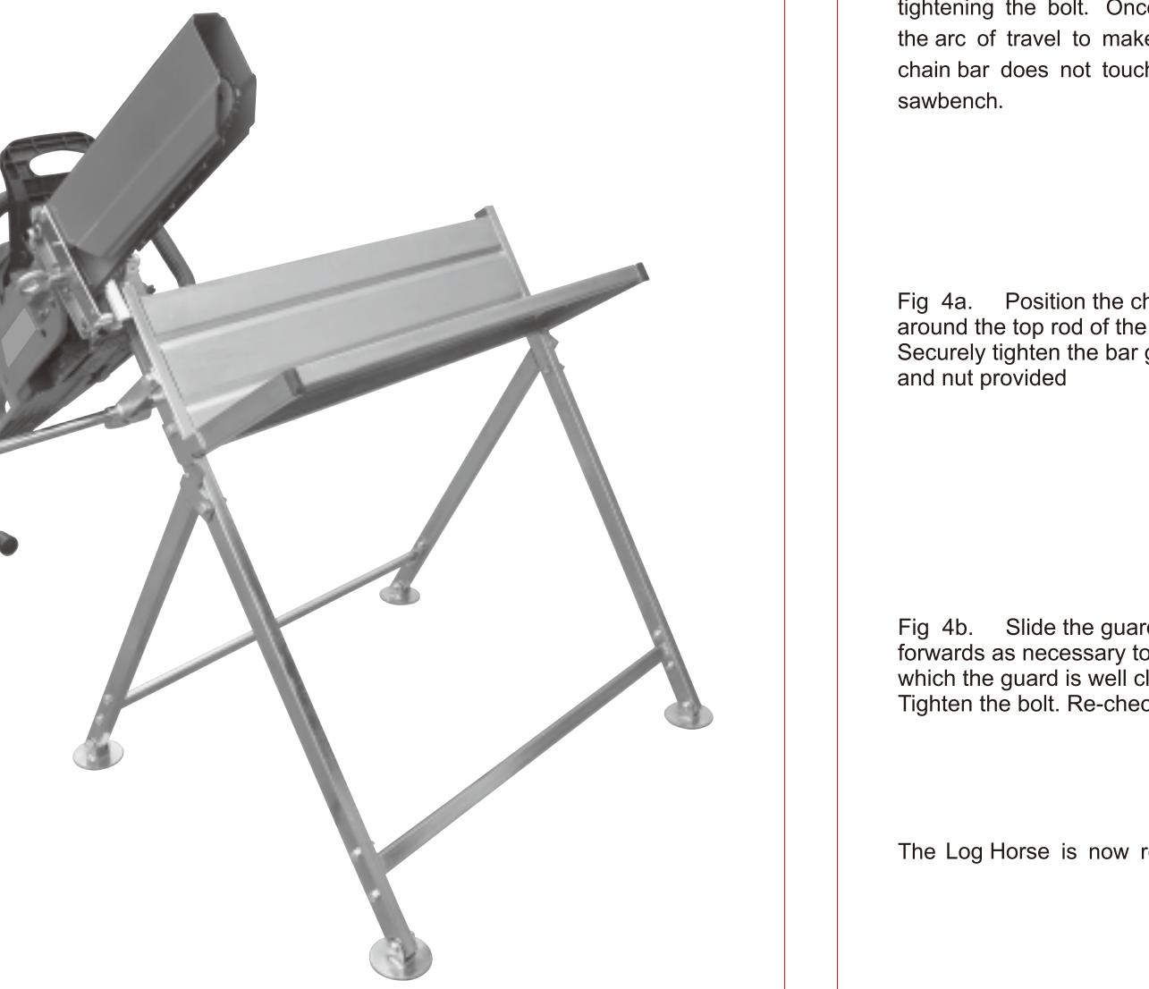
Fig 3. Carefully lower the chainsaw bar into position between the two solid blocks in the pivot clamp and ensure a 2 cm gap between the body of the chainsaw and the clamp. Make sure that the bar is approximately 90 degrees to the clamp and well clear of the chain before tightening the bolt. Once tightened, test the arc of travel to make sure that the chain bar does not touch any part of the sawbench.
