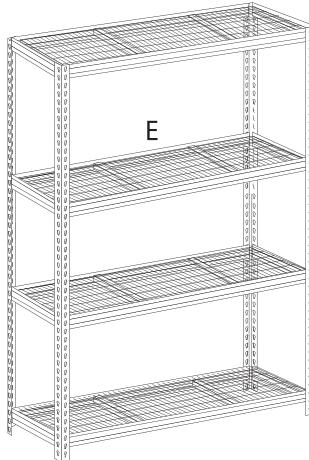
**Step 5: Lay the Wire Shelving (Part E) between the Beams as shown.**
