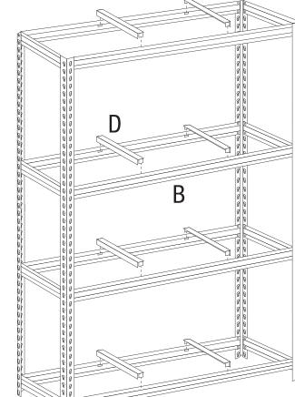
**Step 4: Slot Braces (Part D) into position through the holes provided on the Long Beams (Part B).**
