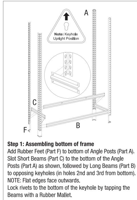
**Step 1: Assembling bottom of frame**
